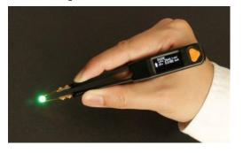
LCR Pro1/Pro1 Plus are able to test additional component parameters such as ESR, DCR, D, Q,  $\theta$ , etc. They can also test diode and indicate polarity and forward voltage/current.
