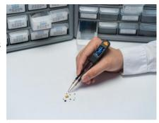
1.0Vrms allows precision measurements of ceramic capacitors with high dielectric constant (K), such as X5R type. 0.2Vrms is specially designed for in-circuit debugging because it is low enough to prevent the silicon chips from being active during measurement.
