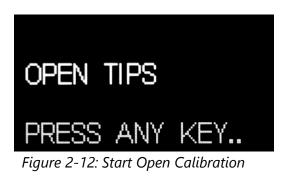
4. Once any button is pressed, Figure 2-13 shows on the display indicating open calibration is in progress.
