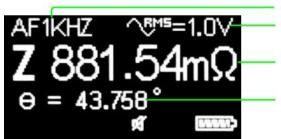
Figure 3-10: Display of Z measurement
