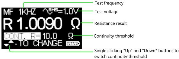
Figure 3-17: Display of Continuity Measurement
