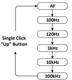
Figure 3-2: Switch Test Frequency by Single Clicking the "Up" Button
