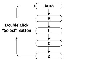
Figure 3-4: Switch Component Type by Double Clicking the "Select" Button
