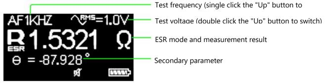
Figure 3-11: Display of ESR Measurement
