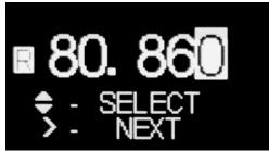
Figure 2-31: Input Digits of Reference Resistance Value
