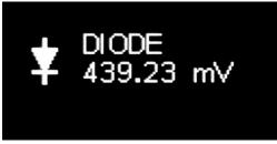
Figure 3-13: Display of Diode Measurement (Good Diode)
