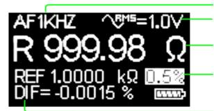
Test frequency (single click the "Up" button to Test voltage (double click the "Up" button to
