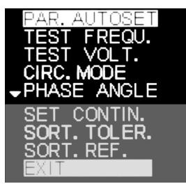
Figure 2-22: Test Parameters Menu
