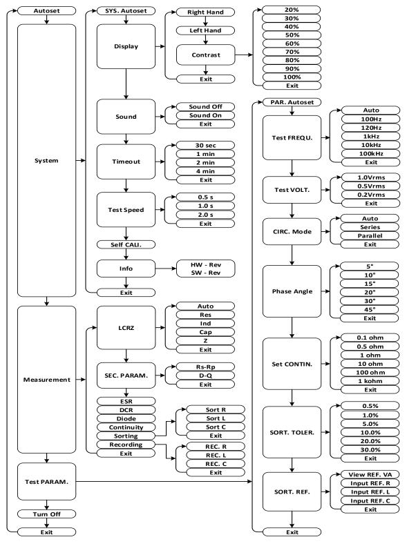
Figure 2-1: Menu Structure Flowchart
