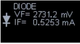
Figure 3-15: Display of LED Measurement
