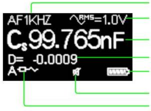
Test frequency (single click the "Up" button to switch)
