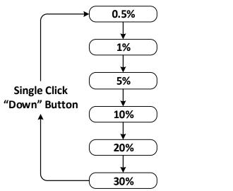
Figure 3-20: Switch Sorting Tolerance Range by Single Clicking the "Down" Button
