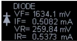
Figure 3-16: Display of LED Measurement (bi-directional LED)
