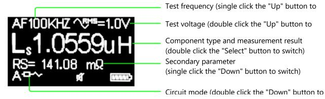
Figure 3-8: Display of L measurement
