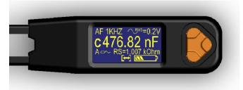
Figure 1-8: Measurement Display
